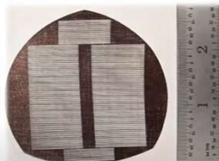
Figure 10: Insert-shape, paper-screen design using 200 μm slits x 20,000 μm slits (Credit: Barker, S.)
